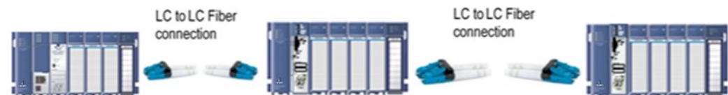
Figure 25: Interconnect using Single-Mode Fiber
