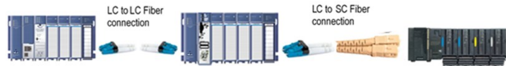
Figure 24: Interconnect using Multi-Mode Fiber
